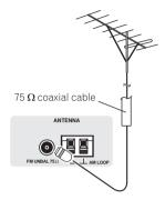
To improve AM reception, connect a 5 m to 6 m (16 ft. to 20 ft.) length of vinyl-coated wire to the **AM LOOP** terminals without disconnecting the supplied AM loop antenna.
